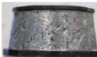
図1 はく離が進展した円すいころ軸受の内輪 Inner ring of tapered roller bearing which flaking had spread
