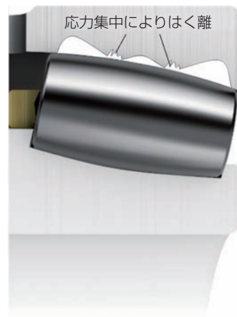
(c) はく離発生箇所 Area of flaking occurrence
