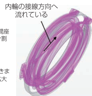
図10(b) 改良間座での空冷エアの流れ Cooling air flow of development designed spacer (Fluid analysis results)
