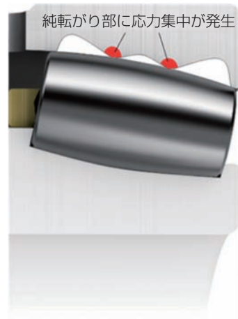
(b) 応力集中発生箇所 Area of stress concentration occurrence
