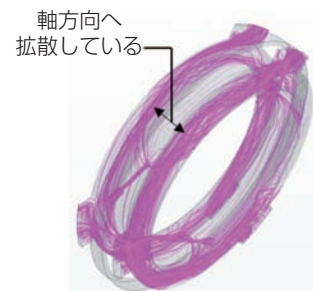
図9(b) 標準間座での空冷エアの流れ Cooling air flow of Standard designed spacer (Fluid analysis results)
