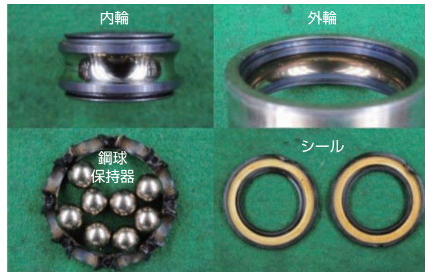
図14 試験後品の外観 Appearance of after test sample
