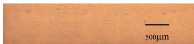
図10 Ti積層造形体の断面組織 Cross sectional microstructure of laser formed Ti compact
