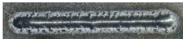
図14 1ライン走査後の概観 Appearance of a laser formed line
