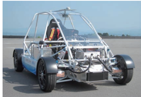
図11 4輪独立の駆動と操舵機能を有する試験車両 Test vehicle with four wheel independent driving and steering
