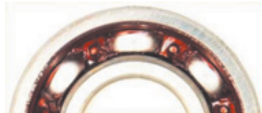
図10 対角凹み保持器（図7）のグリース付着状態 Grease deposition of ball bearing with cage of recessed pocket at diagonal positions (Fig. 7)
