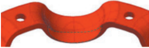
図6 中央凹み保持器 Cage of widely recessed pocket at the center
