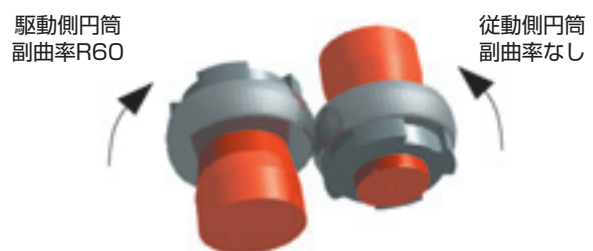
図12 2円筒転がり試験の概略 Schematic diagram of double roller test
