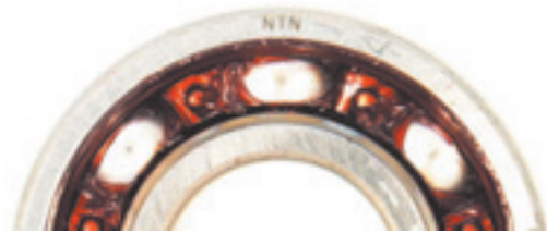
図9 中央凹み保持器（図6）のグリース付着状態 Grease deposition of ball bearing with cage of widely recessed pocket at the center (Fig. 6)
