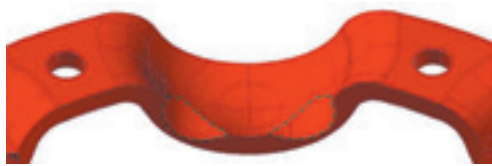
図7 対角凹み保持器 Cage of recessed pocket at diagonal positions
