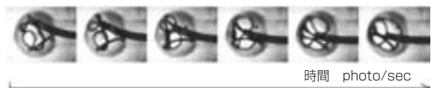
(d) 高速送り出し挿入のコイル展開状態 (1.0mm/s) The photos of the deployed 3D coil by high speed coil insertion
