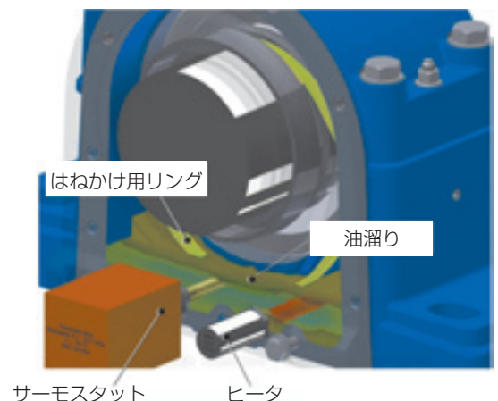
図13 潤滑油の予熱装置設置例 Preheating device of lubricant oil
