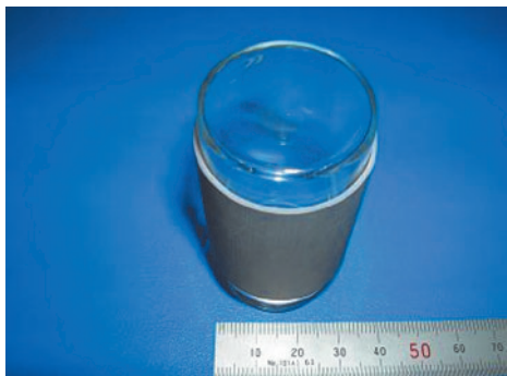
図2 曲面への貼り付け状態 The developed material stucked on curved surface
