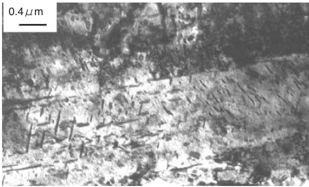
図3 事前熱処理後の組織のT.E.M 顕微鏡検査 T.E.M micrography of the structure after prior heat treatment
