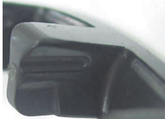
写真2 保持器状況（急加減速試験後） Condition of cage after 2000 (h) of rapid acceleration and slowdown test
