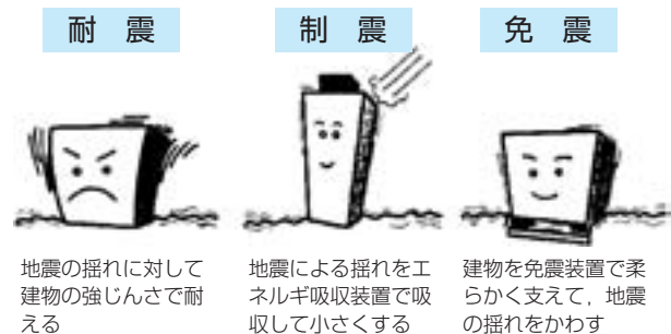
図1 耐震、制震、免震構造の概念 Concept of earthquake resistant structure, vibration control structure, and seismic isolated structure
