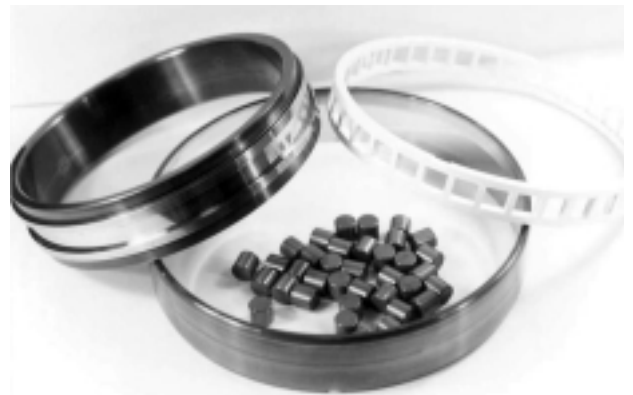
図2 供試軸受外観写真 Cylindrical roller bearings with new materials
