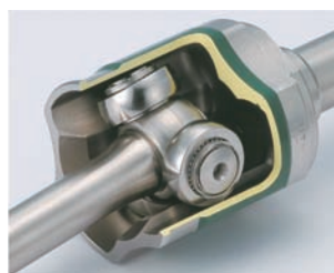
図3 AC-TJの構造 Structure of AC-TJ
