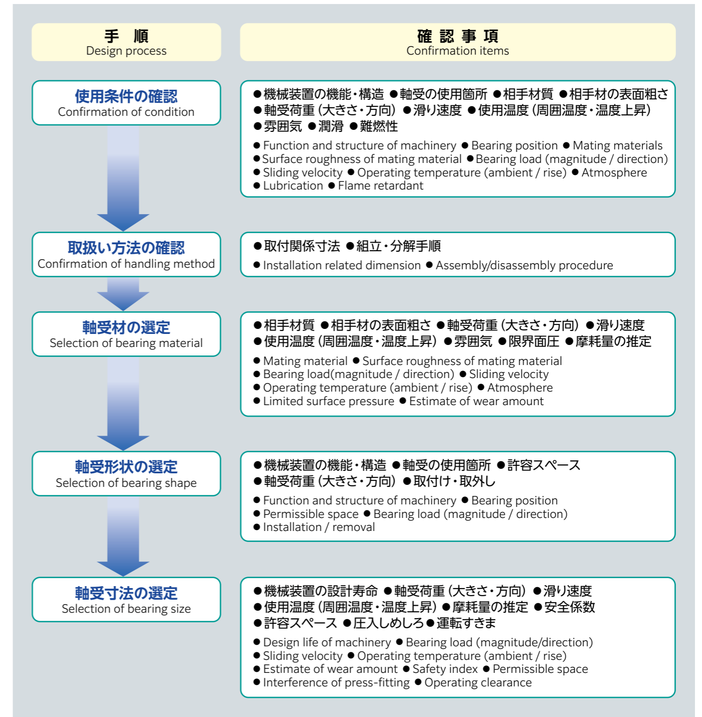
図2-1 樹脂滑り軸受の設計手順 Fig.2-1 Design process for plastics sliding bearings
