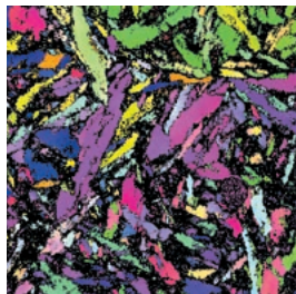
Grain size after nitrocarburizing treatment
