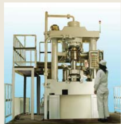
Steel dust solidification system
