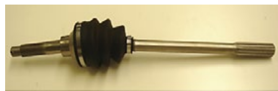
Fig. 5 Exterior of CVJ mounted on Suzulight Van FE
