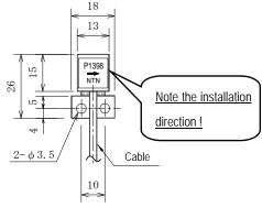
**2**. Outside view (Refer to P59 of operation manual for size) The following diagram is explained about K-ECF25. But the layout of parts is same with K-ECH45.
