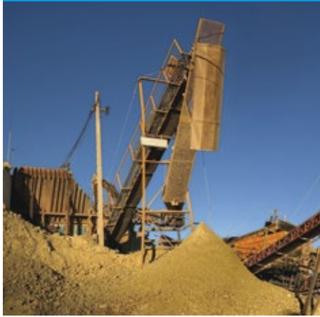
Mining equipment (raw material transportation conveyor)
