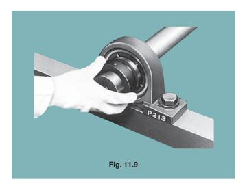
6) Insert a bar into the hole provided on the periphery of the eccentric collar and tap the bar so that the collar turns in the direction of rotation of the shaft (see **Fig. 11.10**).
