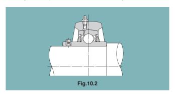
each other. UK type bearing can't support axial load.
