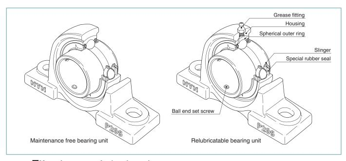
**Mounting system for bearing unit** (Please refer to P56  $\sim$  P59 for Mounting bearing unit on the shaft)
