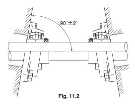
4) Excessive tightening of the mounting bolts may cause the housing to deform. Tightening the bolts to the proper torque can avoid this issue. Also, NTN recommends using a washer with the bolt when mounting the housing as the bolt alone may cause damage to the housing.
