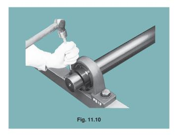
7) Fasten the set screw of the eccentric collar onto the shaft. Recommended tightening torques are given in **Table 11.4**.
