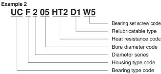
Bearing specifications for heat resistance and cold resistance are shown on **Table 4.3**.
