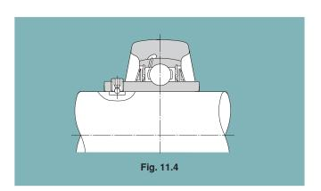
The method of mounting the unit on the shaft is as follows:
