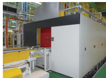
Electrically heated vacuum carburizing furnace (Japan: Kuwana Works)
