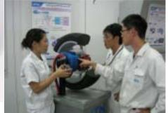
Intelligent In-wheel motor type axle unit
