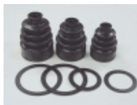
Rubber seals and CVJ boots to be replaced with non-phthalate substitutes
