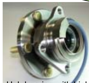
Hub bearing with high resolution rotational sensors
