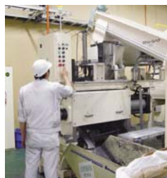
New grinding swarf briquetting machine (NTN Kamiina Corp.)
