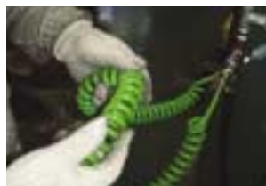
Inspecting for air leaks
