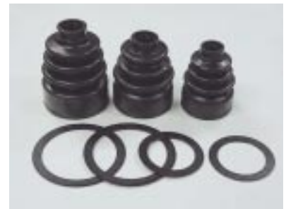
Rubber seals and boots for CVJ that are phthalate ester switchover targets
