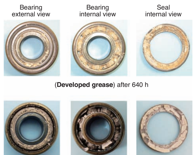
Fig. 13 Internal conditions of bearings after test
