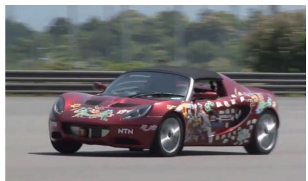
Fig. 11 Driving test with sine-wave steering angle input
