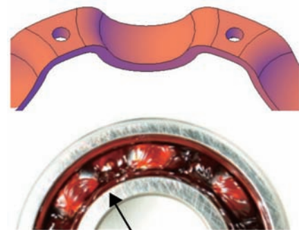
Grease on inner ring seal groove
