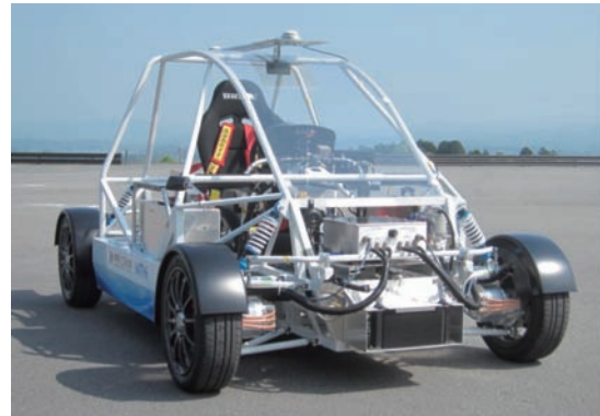
Fig. 11 Test vehicle with four wheel independent driving and steering
