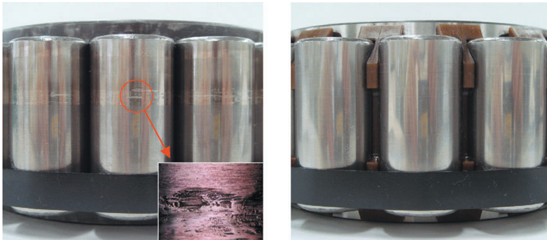
Fig. 8 Bearing condition after test
