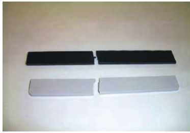
Photo 2 Example of test pieces after evaluation (occurred split and crack)
