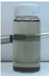
Fig. 9 Recovered horning oil after paper filtration
