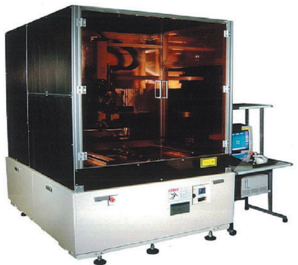
Photo 1 Rib repair system
