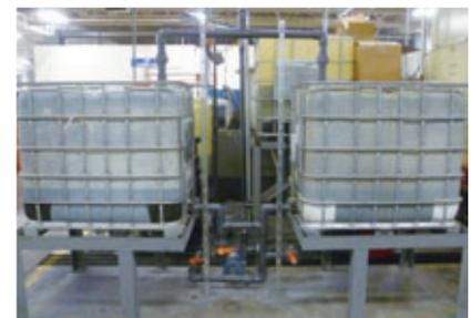
At NTN Bearing Mfg. Canada (CMF), a water circulation system was installed to reduce the amount of water used for tumblers. The company succeeded in reducing annual water use by 1,920 kl and halving the amount of wastewater. ⇒p57
