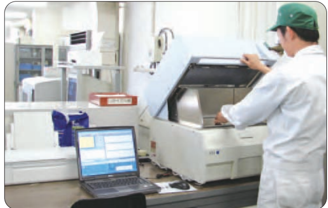
The fluorescent X-ray analysis unit
