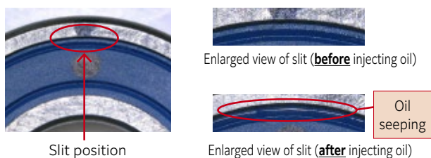
Fig. 11 Performance test of the seal slit
