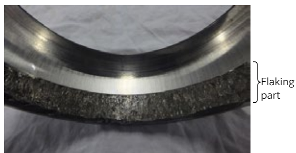
Fig. 9 Outer ring raceway after 300 hours
