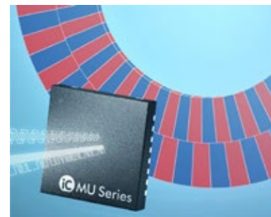
Fig. 11 Image of Combination of iC-MU and Multi Track Magnetic Ring (Conceptual illustration, provided by: iC-Haus GmbH)
