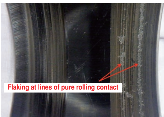
Fig. 6 Flaking on non-slip line
