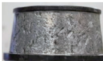
Fig. 1 Inner ring of tapered roller bearing which flaking had spread
