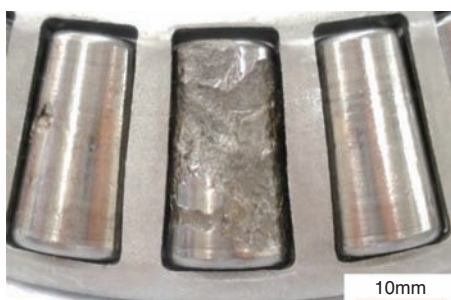
Fig. 13 Test bearing after the continuous test
