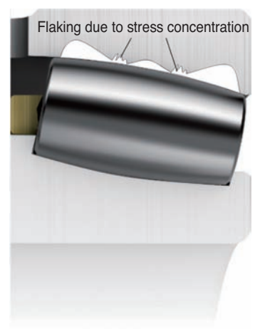
(c) Area of flaking occurrence
