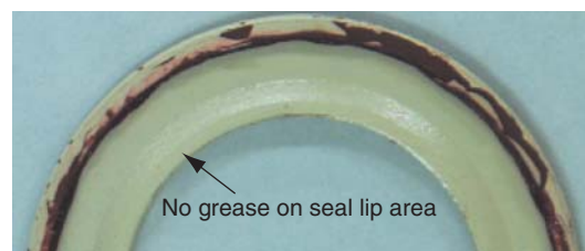
Fig. 16 Adhered grease on the inside of seal with the narrow pocket width cage ( Fig. 14 )
