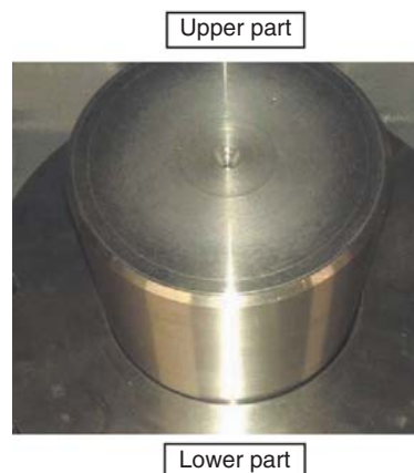
Fig. 18 Gap area after lubricant leak test (no leakage)
