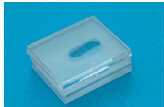
Fig.7 Simultaneous welding of three transparent resin (PMMA) layers
