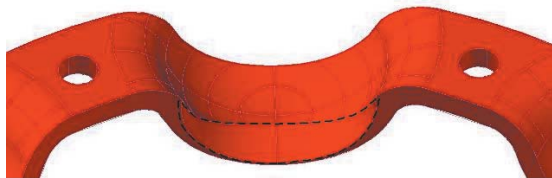
Fig. 6 Design for the widely recessed cage with large chamfer
