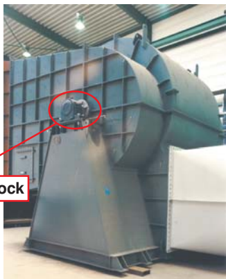
Fig. 1 Application example of oil-lubricated plummer block (large size air blower)
