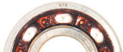
Fig. 9 Grease deposition in bearing using the widely recessed cage ( Fig. 6 )
