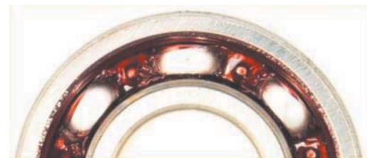
Fig. 10 Grease deposition in bearing using diagonally recessed cage ( Fig. 7 )
