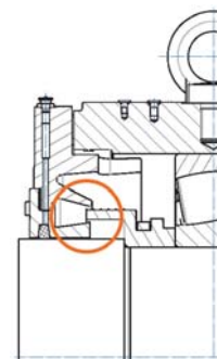
Fig. 16 Labyrinth sealing design of floating side
