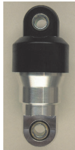
Fig. 15 Compact auto-tensioner for accessory belt
