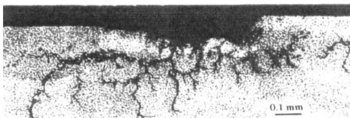
Fig. 6 Cracking on circumferential section of an alternator bearing outer ring (Tamada and Tanaka 12) )
