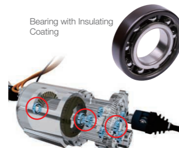
Applied areas in parallel axis e-Axle (red circle)
